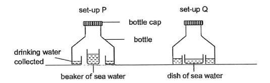
After some time, water droplets appeared on the inner <u>surfaces</u> of both bottles and drinking water collected inside the bottles.
