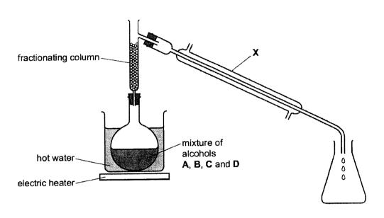
(a) Apparatus X needs to have cold water flowing through it.
