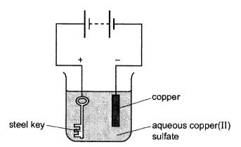
The key does not get coated with copper. Which change needs to be made to plate the key?
