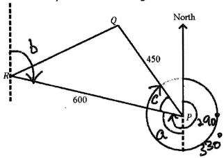
Q is on a bearing of 330° from P and PQ = 450 m. R is on a bearing of 290° from P and PR = 600 m.
