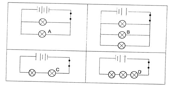
Which bulb(s) would be the brightest?
