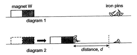
He then repeated the experiment with three other bar magnets, X, Y and Z, of the same length.
