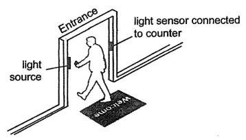
When a person is between the light source and the sensor, the light is blocked. The data recorded by the counter is represented in the graph below.
