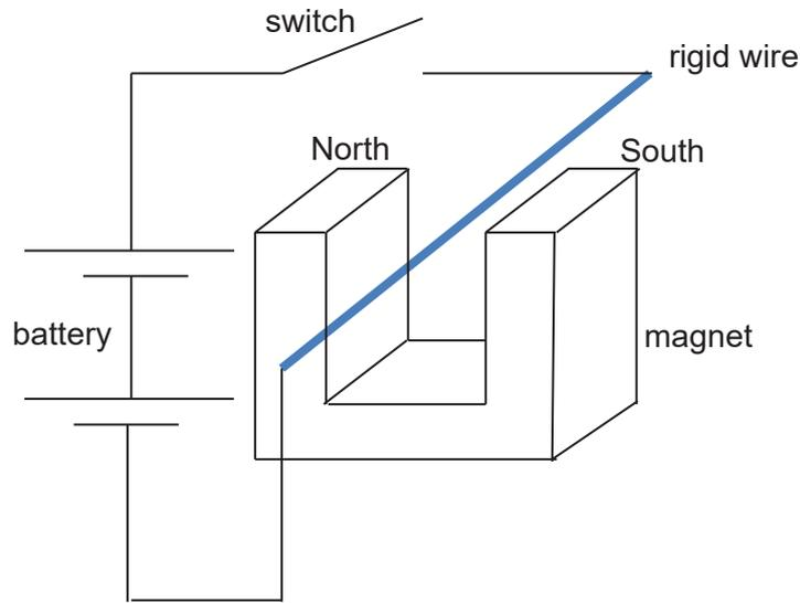
When the current is switched on, there is a force acting on the wire.
