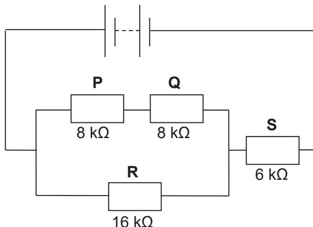
Resistors **P** and **Q** each has a resistance of 8 kΩ. Resistor **R** has a resistance of 16 kΩ and resistor **S** has a resistance of 6 kΩ.
