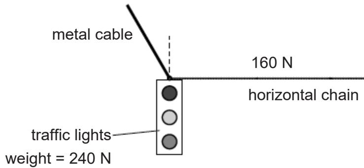
The weight of the traffic lights is 240 N and the tension in the horizontal chain is 160 N.
