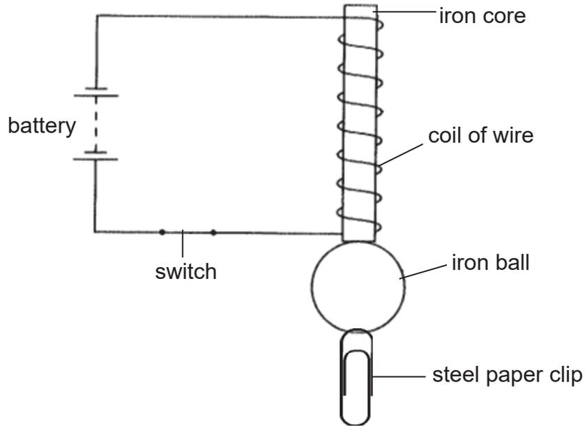
When the switch is closed, an iron ball is attracted to the iron core. The steel paper clip is attracted to the iron ball.
