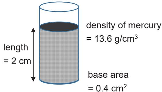
The cross-sectional area of the cylinder is 0.4 cm<sup>2</sup>.
