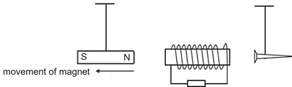
What is the direction of the current flowing through the fixed resistor and the direction that the iron nail moves?
