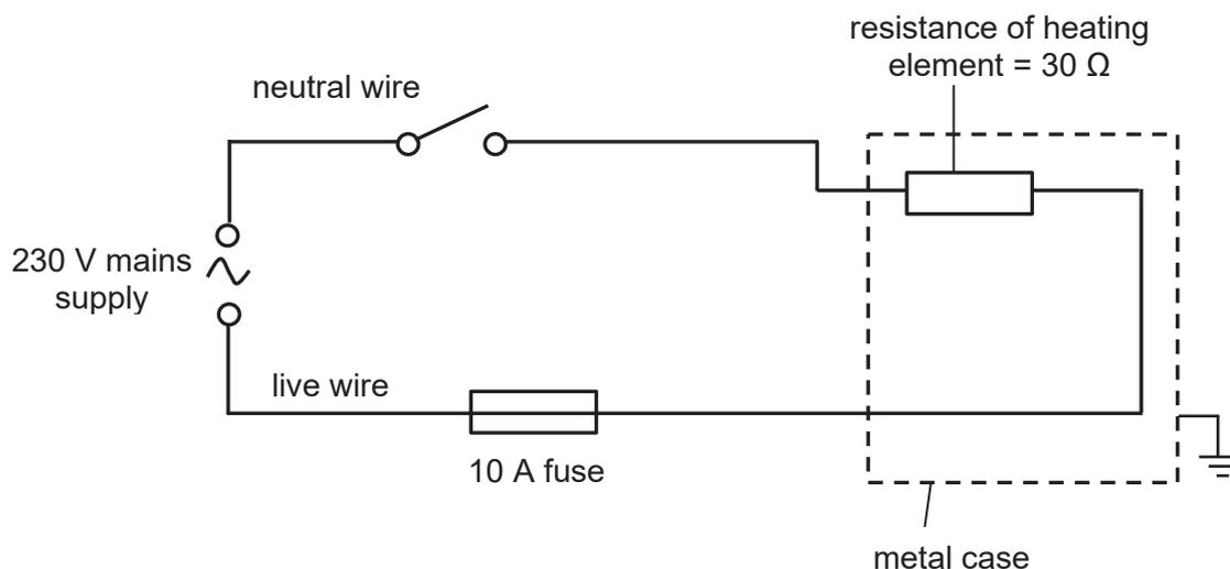
What is the fault in this circuit arrangement?
